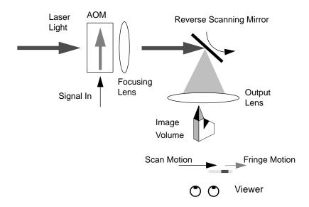
Typical numbers are as follows: hogels are 4K samples wide, with fringelets of 512 samples. (Compression ratio is therefore 8.) Using this method of optical fringelet decoding in a viewer-plane geometry, the current 36-MB MIT display can produce an image that is 8 times larger (in a combined image-volume and view-angle sense) without requiring additional bandwidth. In general, optical replication works best for viewer-plane geometry since hogel widths can be larger.
